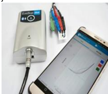
Figure 5. A proposed portable modified HNTs screen printed electrode for FEN electrochemical detection
